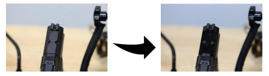
Step 3: Using the Socket head cap screws in the MNT HDWR bag, secure the foundation plate of the OuterImpact mount to the slide with 15 in/lbs of torque.
